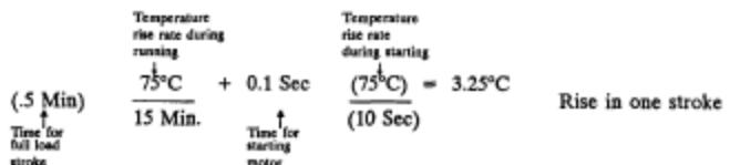
The above example is simplistic and is given only to show that the motor temperature rise associated with stroking the valve is insignificant. However, applications that allow the motor to draw locked rotor current until the system or valve stabilizes must be addressed. A 5 second duration at locked rotor current will result in a temperature increase of ≤ 37.5°C. It should be noted that continual diagnostic testing will increase motor temperature and decrease output torque and thrust.
