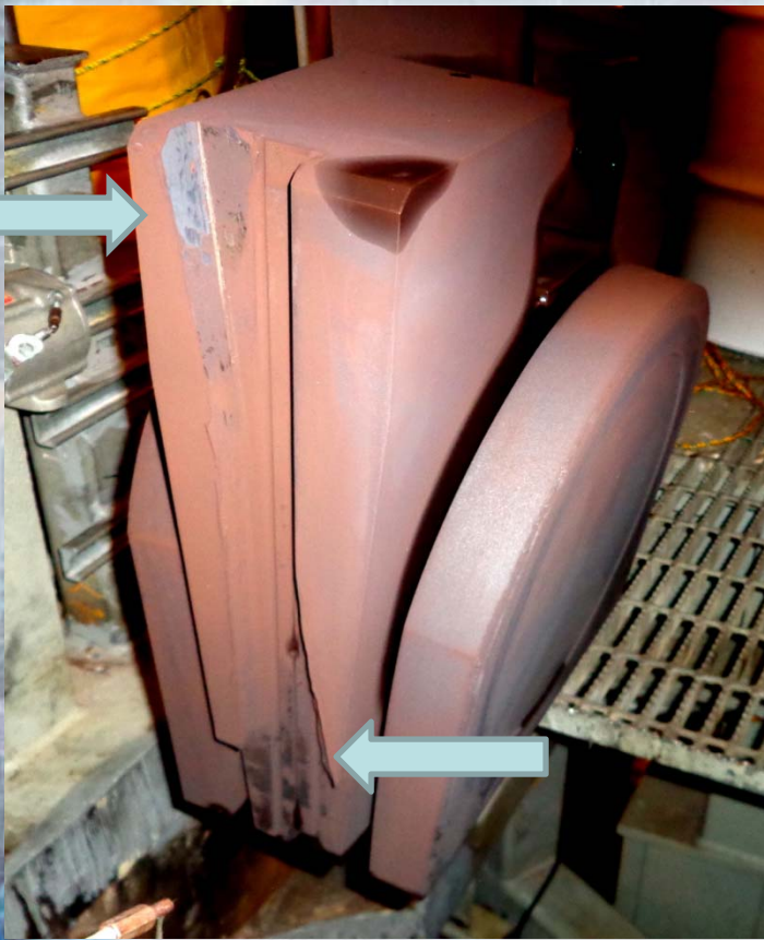
Damaged Disc Guides
